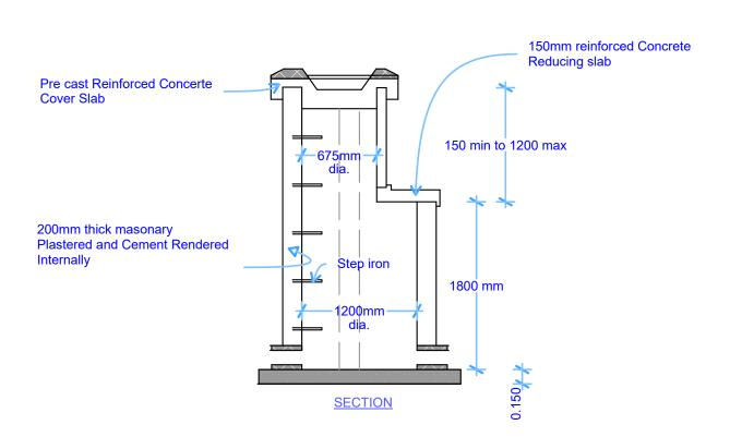
Step iron to BS 1247,staggered 150mm from each side of centerline and spaced @ 300mm vertically
